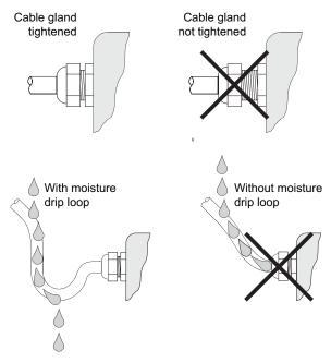
Careful cable routing and sealed ports can help prevent water intrusion.
