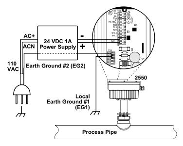
Connect a local earth ground to the TS5 terminal strip as illustrated (EG1). If the cable from power source to the 2550 is less than 200 ft./61m, EG2 is an acceptable alternative. Using both EG1 and EG2 is always the best system.
