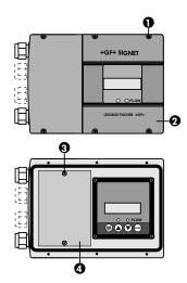
All wiring is installed through the watertight ports in the meter. Wrap threads with sealing tape before threading into sockets.
