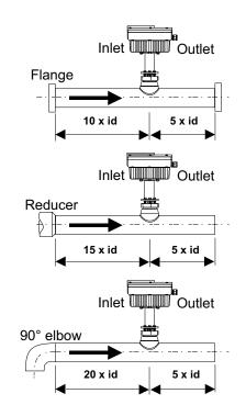
Measure and record the interior diameter of the pipe. This value will be required to calibrate the 2550.
