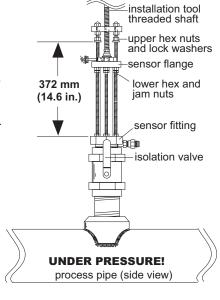
**D.** Wearing safety face protection, loosen the upper hex nuts and raise to 372 mm (14.6 in.) from top of sensor fitting to bottom of upper hex nuts/lock washers. **CAUTION!** This measurement is critical to maintain watertight seal in sensor while allowing clearance to close the isolation valve.
